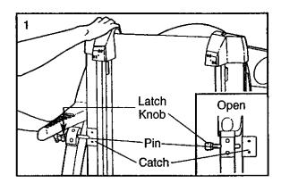
Hold the treadmill firmly with both hands, and lower the treadmill to the floor. Do not drop the treadmill frame to the floor. CAUTION: To decrease the possibility of injury, bend your legs and keep your back straight.
